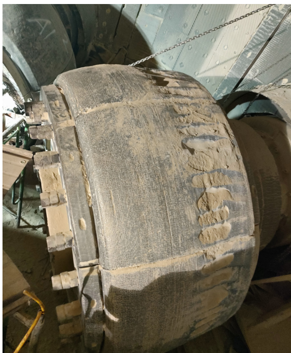
Figure 2. HiCr rollers with hard facing solution.
